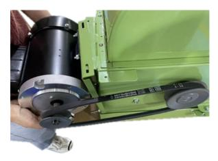
3 Use a straight edge to align the pulleys by sliding the motor to the left or right and then tighten the two screws into the motor mount bracket.
