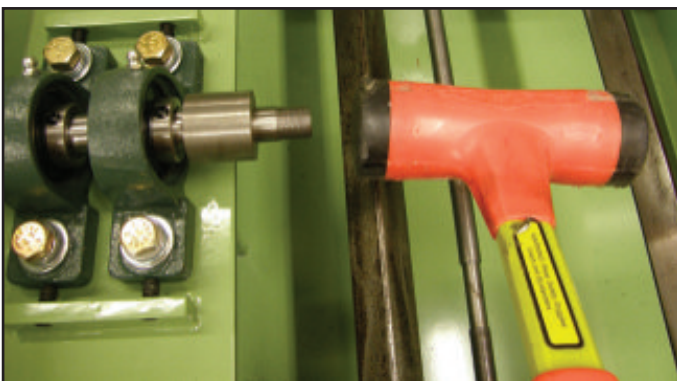
USE A RUBBER Mallet, NOT A HARD HAMMER
