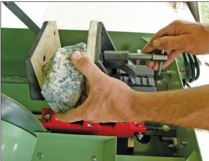
WORKPIECE MUST BE HELD FIRMLY IN VISE.
