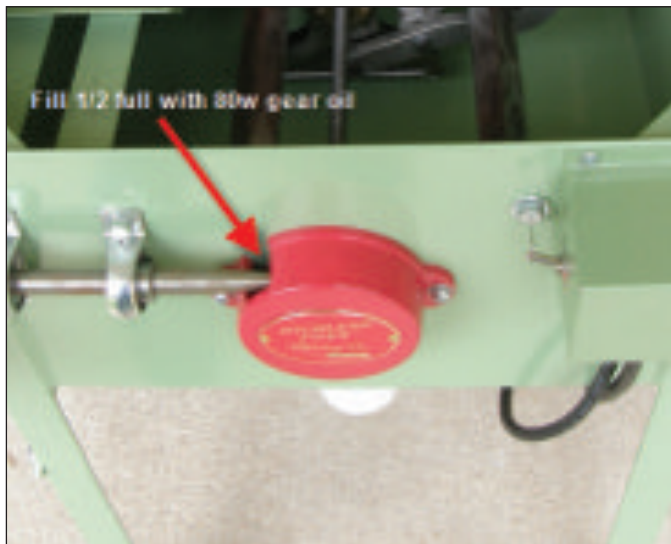
FILL GEAR BOX 1/3- 1/2 FULL WITH 80W GEAR OIL
