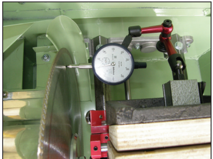
MEASURE FROM SAME POINT OF BLADE
