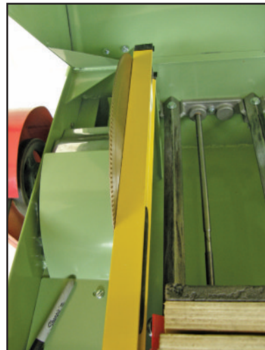
A STRAIGHT EDGE IS USED TO CHECK BLADE STRAIGHTNESS.
