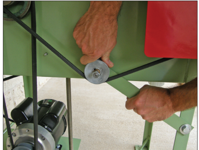
THE IDLER ARM IS ADJUSTED TO TENSION POWER FEED V-BELT.
