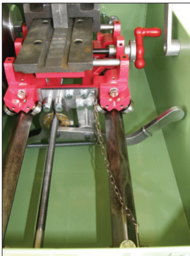
THE AUTOMATIC CUT OFF TRIP CHAIN IS ADJUSTED FOR LENGTH OF CUT.
